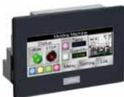
Touch (relay output) (photo: FT1A-*12RA-B)
